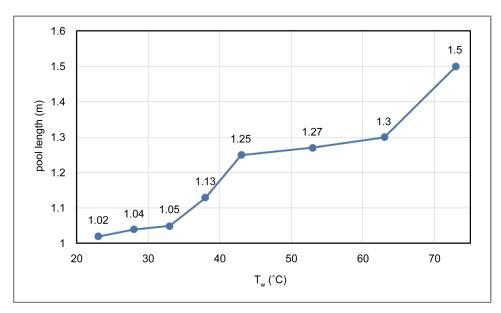
Figure 4. Varying pool length with increasing inlet water temperature.
