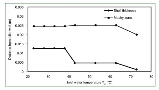
**Figure 6.** Solid shell thickness and Mushy zone at exit section for a range of inlet water temperature  $T_w$ .
