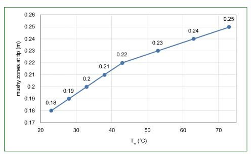
Figure 5. Varying mushy zone thickness against inlet water temperature.
