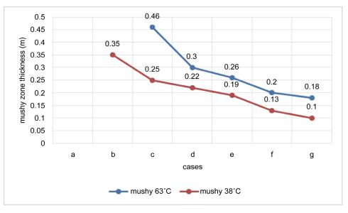
Figure 8. Mushy zone thickness at solidification tip for different secondary cooling intensity cases.
