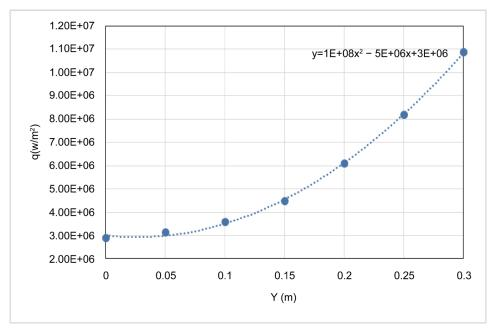
**Figure 2.** Heat flux versus mould height for  $T_w = 23$  °C.
