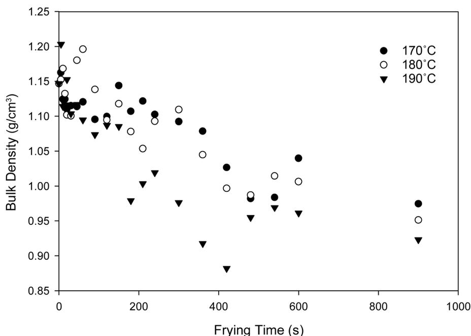
**Figure 1.** Bulk density as a function of time for de-boned chicken meat deep-fat fried at  $170^\circ\text{C}$ ,  $180^\circ\text{C}$ , and  $190^\circ\text{C}$ .
