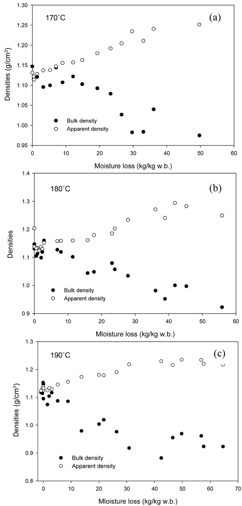
Figure 3. Bulk and apparent densities as a function of moisture loss during deep-fat frying of de-boned chicken meat.
