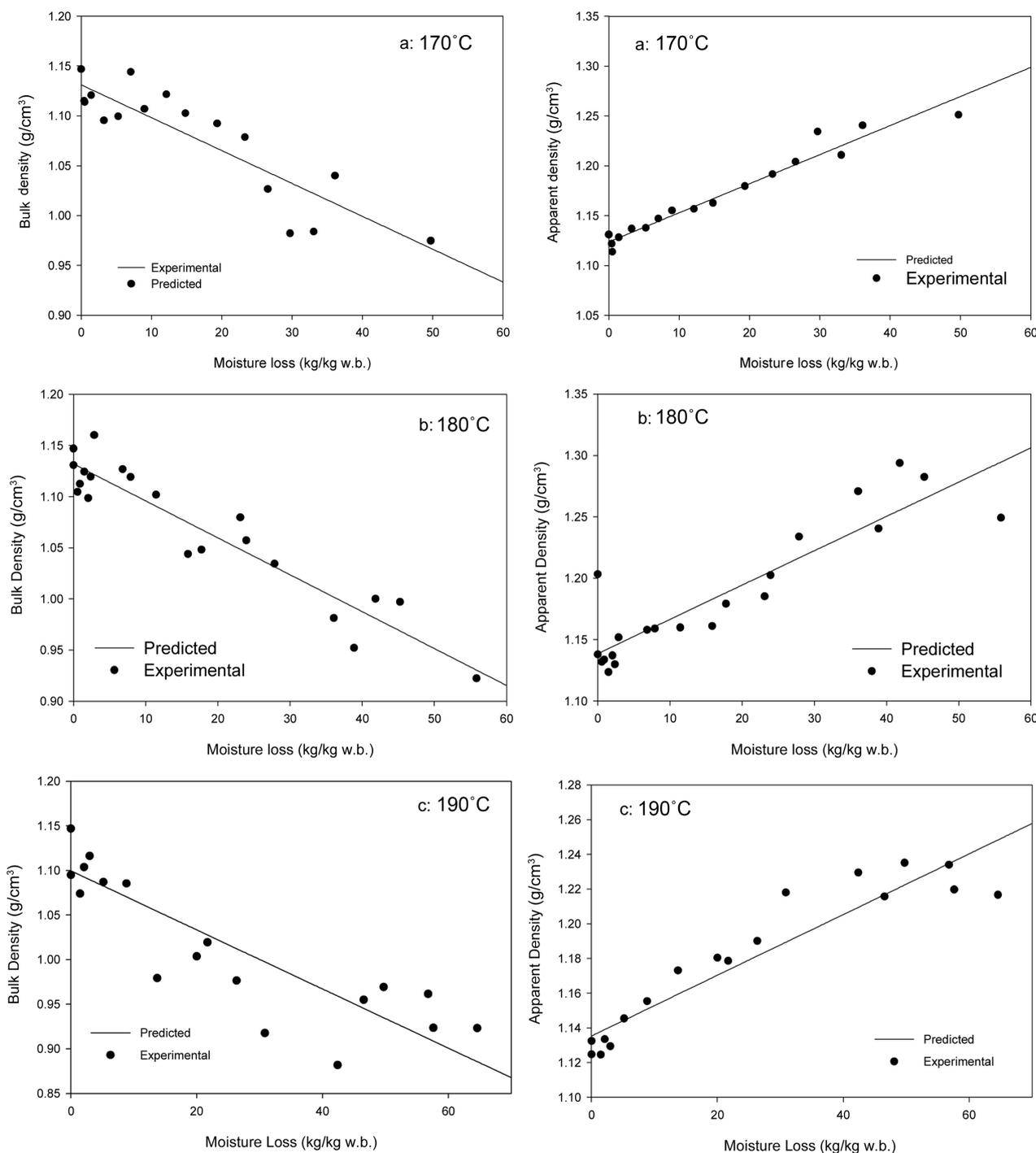
**Figure 4.** Experimental and predicted densities (bulk and apparent) of de-boned chicken meat as a function of water loss fraction during deep-fat frying.
