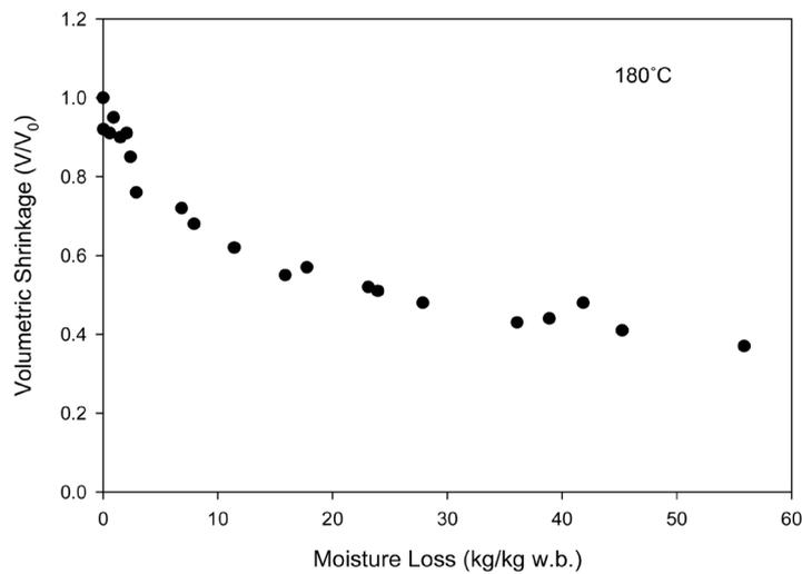
Figure 6. A typical apparent volumetric shrinkage of as a function of moisture loss for FOT 180°C.
