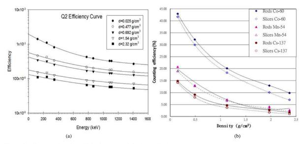
Figure 2. Efficiency of (a) three HPGe detectors and (b)  $4\pi$  scintillation detectors.
