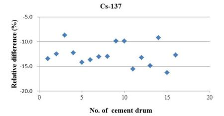
Figure 5. Comparison measurement of concrete drums with homogeneous radioactivity distribution.
