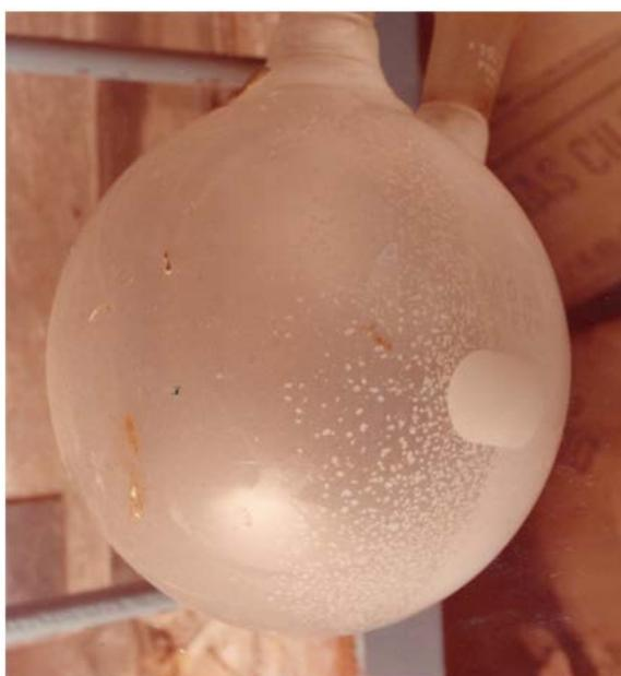
**Figure 8.** Crystals of  $\text{Sn(II) Cl}_2$  deposited on the inner walls of the condenser.
