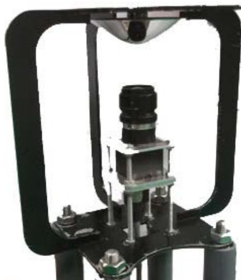
Figure 2. Omnidirectional vision system: parabolic/conic mirror facing downwards and a color camera facing the mirror.
