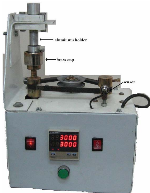
Figure 2. Wear device which was used in this investigation.
