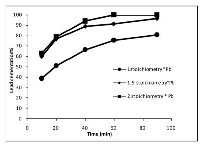
Figure 1. Effect of Al addition on lead cementation, T = 50°C, pH<sub>in</sub> = 4, Stirring Velocity = 100 rpm.
