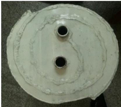
Figure 3. Completed heat exchanger.
