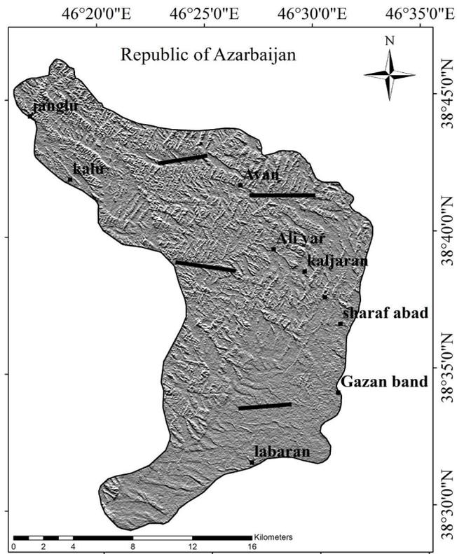
Figure 4. E-W directional filter and extracted lineaments.
