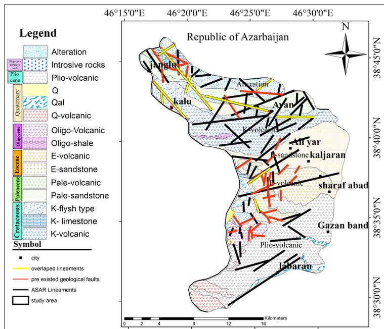
Figure 8. Map of previously verified faults by geological survey of Iran.
