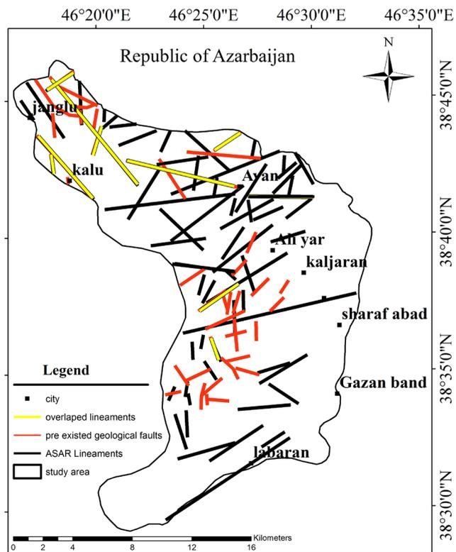
Figure 7. Lineaments map generated after directional filtering operation.
