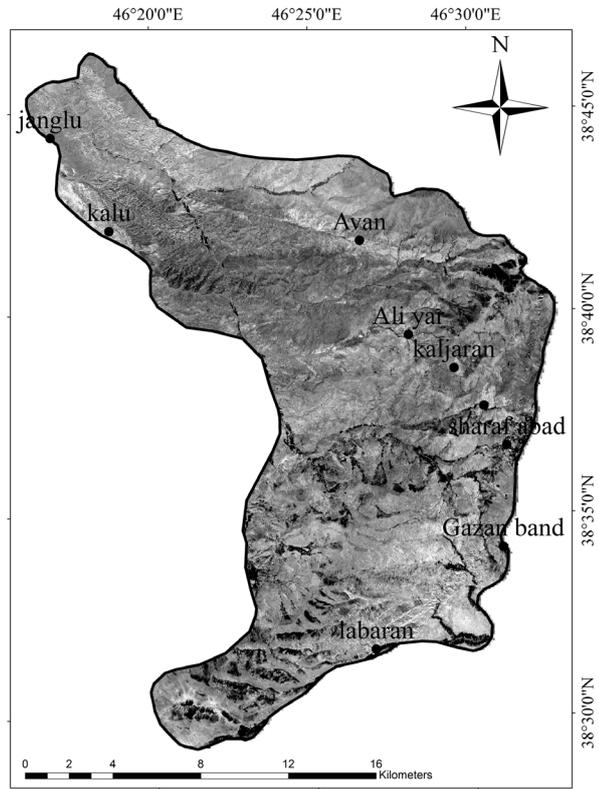
**Figure 17.** Band ratio of B2/B1 for ferric-iron oxide minerals.
