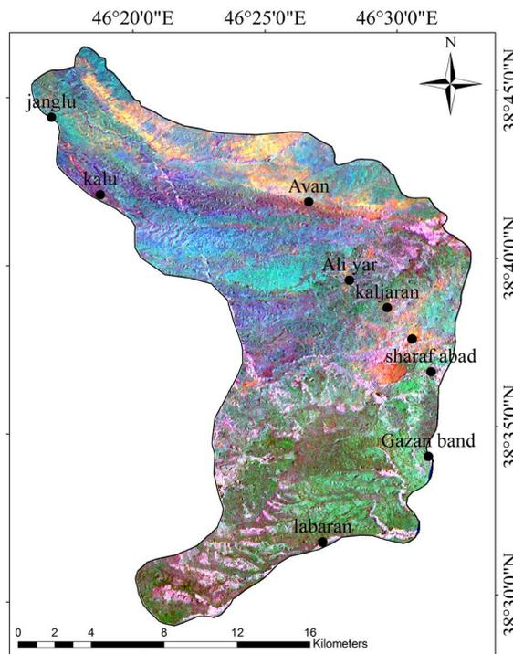
**Figure 20.** Color composite image of band ratios by applying advanced argillic alteration to red, phyllic alteration to green and propylitic alteration to blue (R:G:B = 4/6:5/6:5/8).
