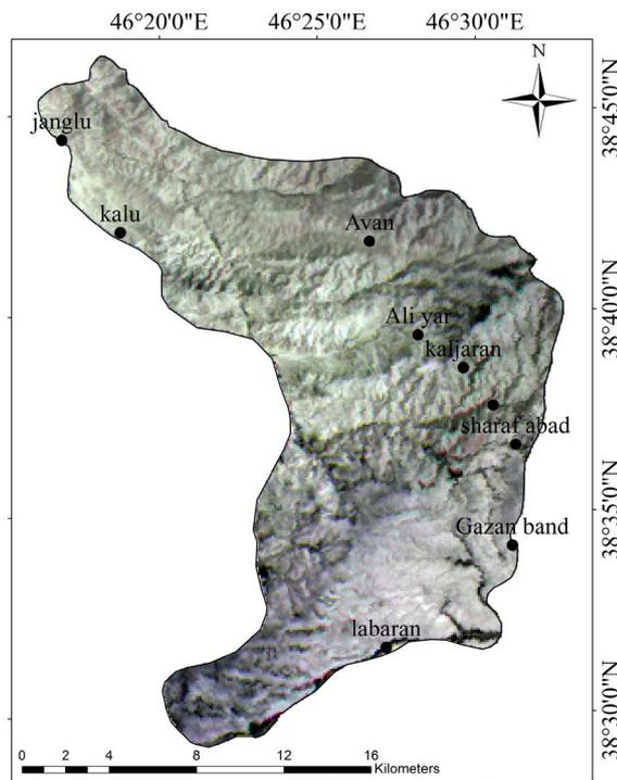
**Figure 13.** Color composite in TIR region (R: 14, G: 12, B: 10) to identify mafic-to-ultramafic units and quartz rich felsic units.
