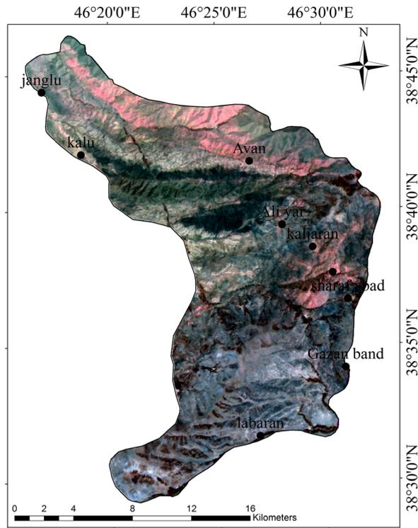
**Figure 12.** In the SWIR false color image, advanced argillic (alunite, kaolinite) alteration and phyllic alteration (sericite, smectite) appear as pink, propylitic alteration (chlorite, epidote) appears as green and calcareous units appear as yellow.
