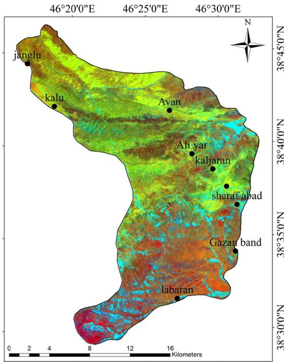
**Figure 19.** VNIR and SWIR color composite ratio images created by applying band ratio B2/B1, B4/B9, B3/B2 to red (R), green (G), and blue (B) (R:G:B) that yellow color represents the presence of hydrothermal alteration.
