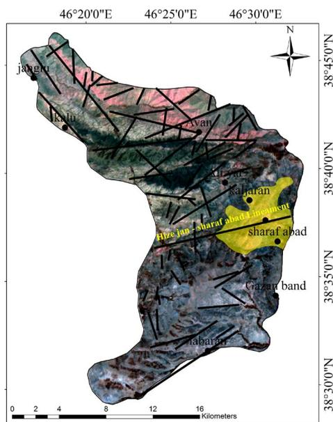
Figure 10. integration of ASAR-ASTER imagery and extracted lineaments (Hizejan-sharafabad Lineament) and relation with Alteration zone map (Yellow polygons).
