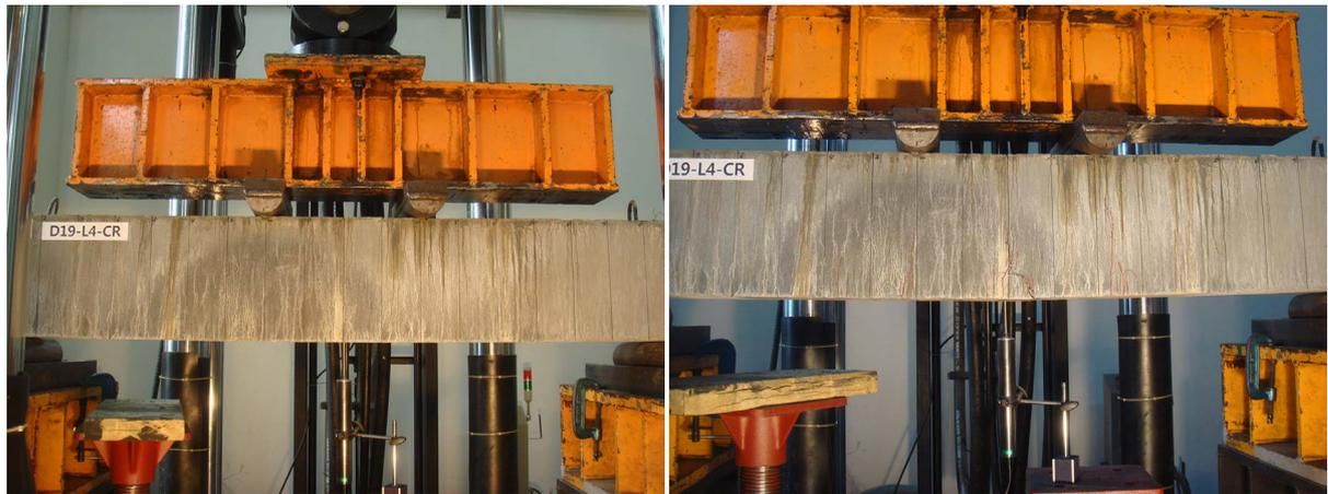
(a) Before flexural strength test
