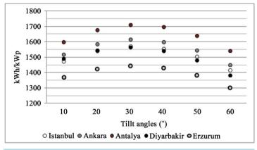
Figure 4. The final PV system yield related to the different tilt angles.
