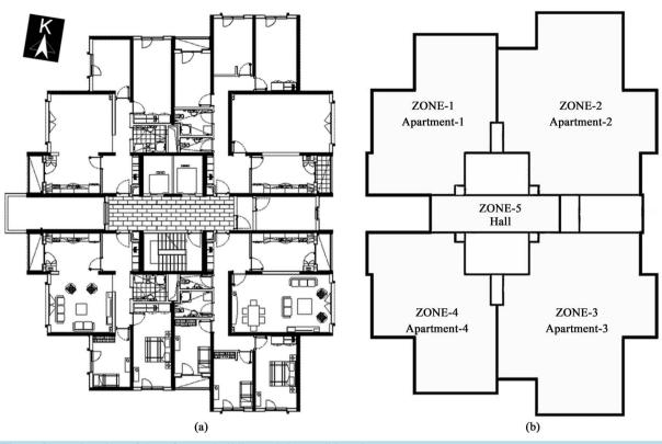
Figure 2. (a) Plan view of the reference building and (b) conditioned zone areas.
