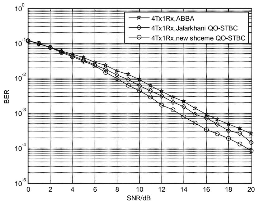
**Figure 2.** BER versus SNR of three QO-STBC schemes.
