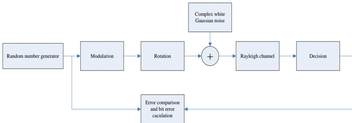
**Figure 1.** Simulation block diagram of QO-STBC.
