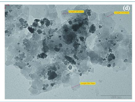
**Figure 2.** SEM micrographs of (a) without *i.e.* 0% NC and (b) with 1.75% NC and TEM images of composite loaded with 1.75% NC ((c) and (d)).
