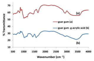
Figure 1. FTIR spectrograms of neat guar gum and acrylic acid guar gum.
