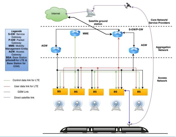
Figure 1. GSM-R and LTE-R architecture.
