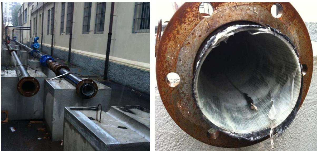
**Figure 8.** Field test at the Armi station in Milano and a close-up of the pipe relined. A 30 m, 30 cm ID steel pipe 30 m has been relined with the vinyl ester acrylate resin, filled with aqueduct water and, after 24 h the water has been sampled and analysed as described in the text.
