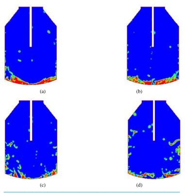
Figure 4. Phase distributions after 5 s from the start of blowing. Blowing condition: (a) top, (b) combined-center, (c) combined-lateral, (d) full combined.
