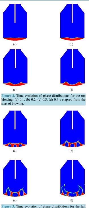
**Figure 3.** Time evolution of phase distributions for the full combined blowing. (a) 0.1, (b) 0.2, (c) 0.3, (d) 0.4 s elapsed from the start of blowing.
