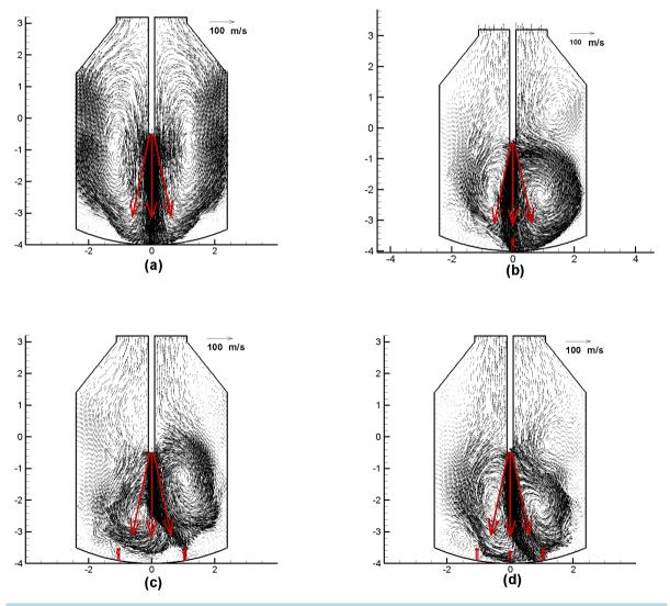
Figure 1. Velocity vectors after 1 s from the start of blowing. Blowing condition: (a) top, (b) combined-center, (c) combined-lateral, (d) full combined.
