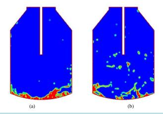
**Figure 5.** Phase distributions after 7 s from the start of blowing. Blowing condition: (a) top, (b) full combined.
