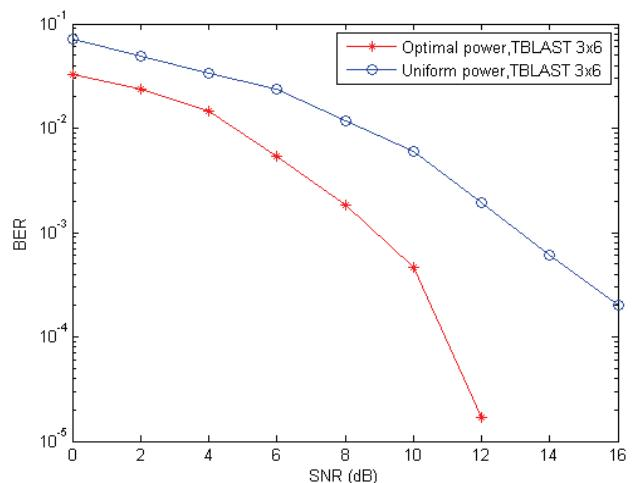
**Figure 3. BER Performance comparison: OPL versus equal power allocation.**
