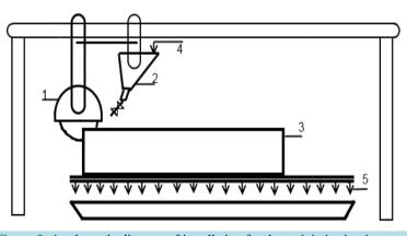
Figure 3. A schematic diagram of installation for dust minimization in stone quarry. 1. Stone-cutting instrument; 2. Funnel for naphthenate solution supply; 3. Stone; 4. Naphthenate solution; 5. Vessel for gathering dust-naphthenate mixture.
