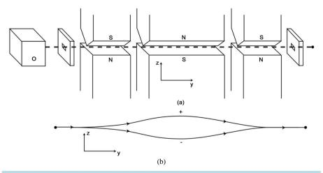
Figure 2. (a) An imagined modification of a Stern-Gerlach apparatus; (b) The paths of spin 1/2 particles.
