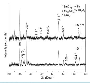
Figure 1. XRD of SmCo/FeCo/SmCo films with different thickness and heat treatment.
