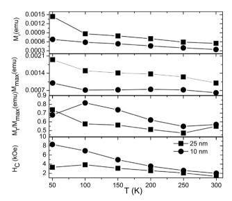
Figure 3. Magnetic properties behavior of SmCo/FeCo/SmCo films with different soft phase thickness 10 and 25 nm.
