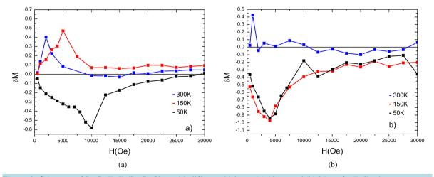
Figure 4.  $\delta M$  curves of SmCo/FeCo/SmCo films with different thickness (a) 10 nm and (b) 25 nm for FeCo phase.
