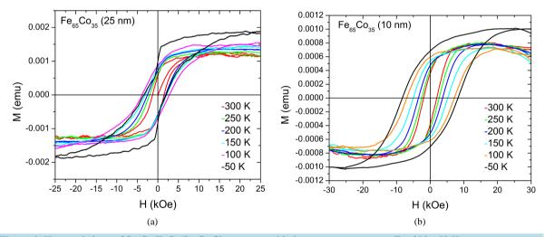
Figure 2. Hysteresis loop of SmCo/FeCo/SmCo films measured in low temperature range T = 300 - 50 K.
