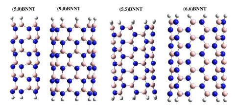
Figure 1. The fully optimized structures of (5,0), (9,0), (5,5) and (6,6) BNNTs. Nitrogen atoms (blue), Boron atom (pink) and hydrogen atoms (white).
