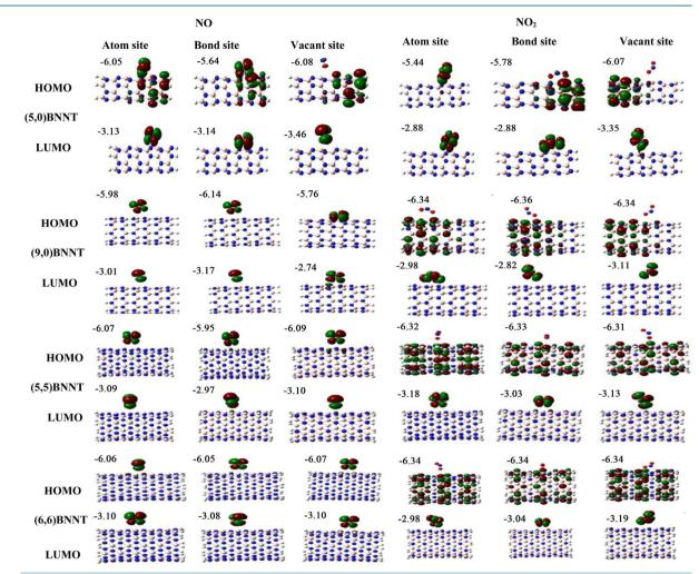
Figure 3. HOMO and LUMO molecular orbitals of adsorbing NO and  $NO_2$  gas molecules on the pristine (5,0), (9,0), (5,5) and (6,6) BNNTs. Energies of HOMO and LUMO are listed above the molecular orbitals and are given by eV.
