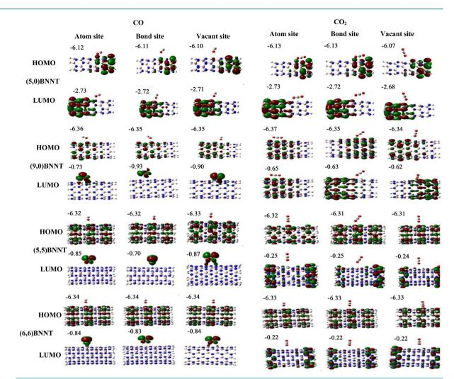
Figure 2. HOMO and LUMO molecular orbitals of adsorbing CO and  $CO_2$  gas molecules on the pristine (5,0), (9,0), (5,5) and (6,6) BNNTs. Energies of HOMO and LUMO are listed above the molecular orbitals and are given by eV.
