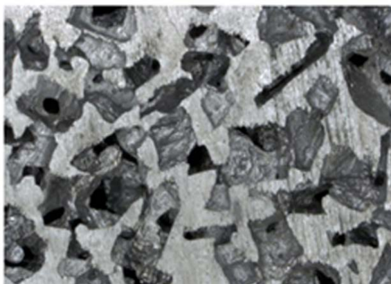
Figure 1. SEM image of the low porosity aluminum foam structure.
