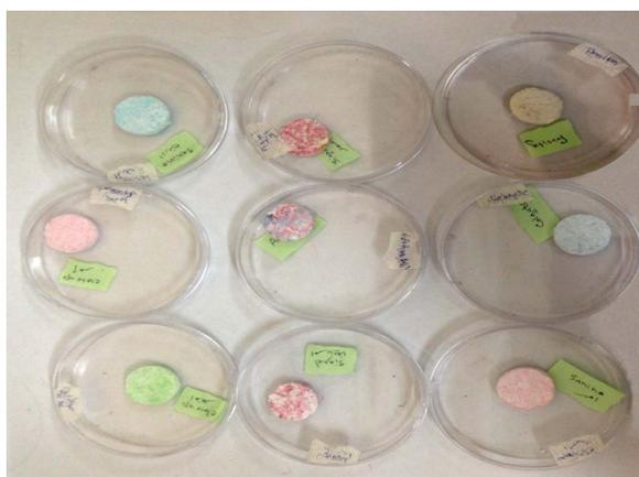
**Figure 1.** Shows samples covered with nuclear track detector (CR-39).
