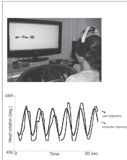
**Figure 4.** Presents the head tracking task and presents synchronous plots of the target cursor motion and user head rotation for a typical tracking task.
