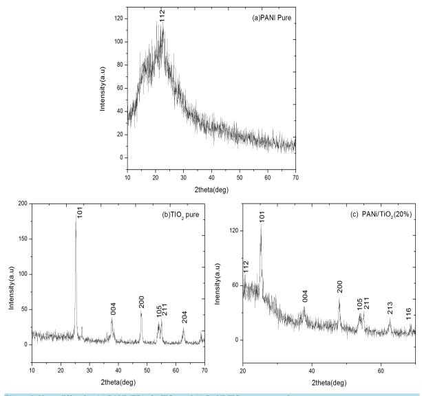
Figure 2. X-ray diffraction (a) PANi (EB), (b) TiO<sub>2</sub>, and (c) PANI:TiO<sub>2</sub> nanocomposite.
