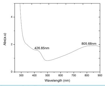
Figure 5. The absorption spectrum of polyaniline (EB) in the visible spectrum.
