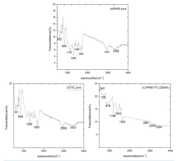
Figure 4. FTIR spectra of (a) PANI (EB), (b) PANI:TiO<sub>2</sub>, and (c) TiO<sub>2</sub>.
