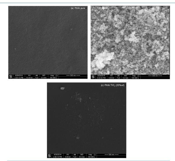
Figure 3. FESEM morphology of (a) pure PANI, (b) pure TiO<sub>2</sub>, and (c) PANI:TiO<sub>2</sub> (20% wt).
