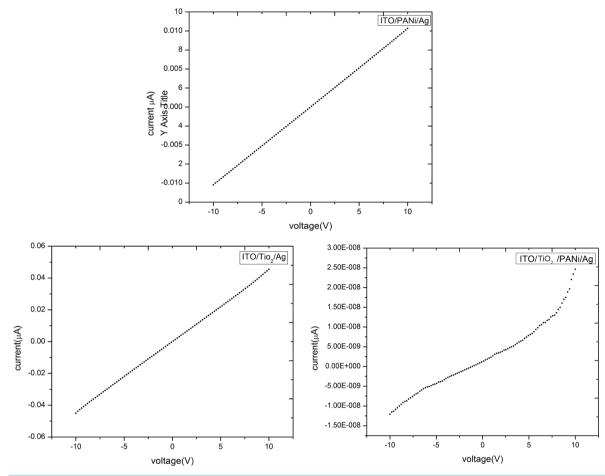
Figure 6. I/V characteristic of the sandwich-type structure of PANI, TIO<sub>2</sub>, and ITO/TiO<sub>2</sub>/PANI/Ag.
