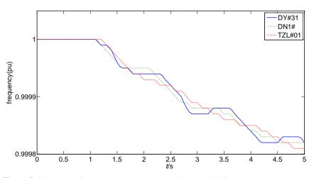
Figure 3. The system frequency response curves when cut DJP#2 generator.
