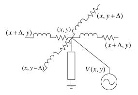
Figure 1. A distributed discrete power system.
