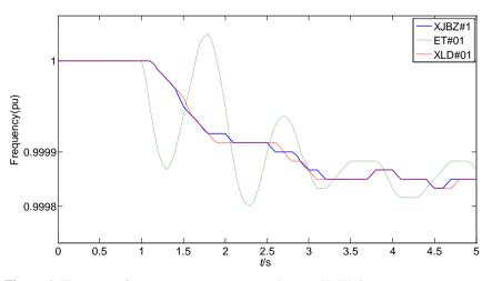
Figure 6. The system frequency response curves when cut HMK#2 generator.
