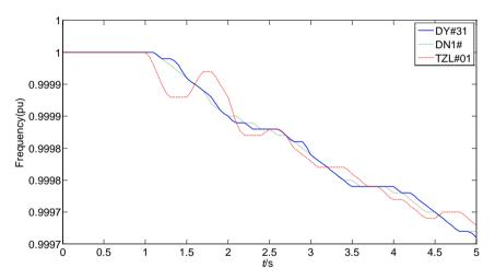
Figure 2. The system frequency response curves when cut PT#02 generator.
