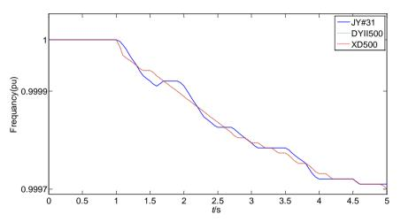
Figure 5. The frequency response curve when cut WWS81 generator.
