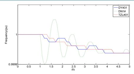
Figure 4. The system frequency response curves when cut FYB#2 generator.
