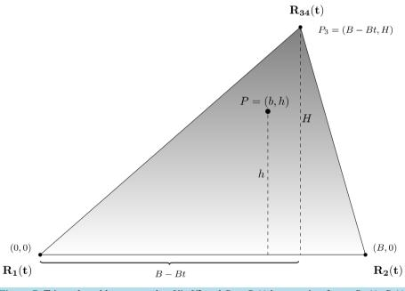
**Figure 7.** Triangular table supported at V1; V2 and  $P_3 = P_3(t)$  has reaction forces  $R_{34}(t)$ ;  $R_1(t)$  and  $R_3(t)$ .
