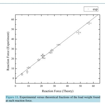
mental fraction reaction force is the slope of a linear fit such as those in Figure 12 (reaction forces versus load weights). The y-error bars on the data are uncertainties from the resulting linear fits, such as in Figure 12. The x-error bars are from calculations of the uncertainties of the positions of the load weights, limited by the apparatus.
