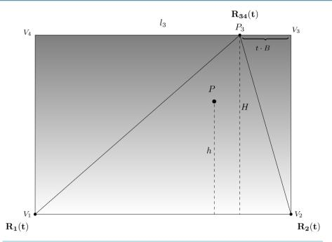
**Figure 6.** In this view from the top of the rectangular table described before, reaction force  $R_{34}(t)$  on segment  $l_3$  replaces forces  $R_3$  and  $R_4$  for some t in the interval [0; 1].
