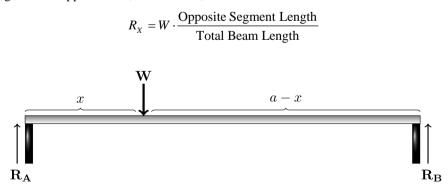
Figure 1. The beam case consists of a two legs table and a load W located at distance x from one of the legs.
