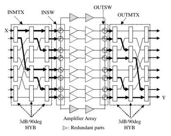
Figure 6. Block diagram of MPA.
