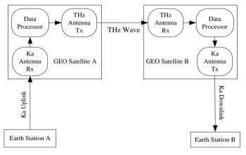
Figure 2. Block diagram of MODE 1 (GEO-GEO link).
