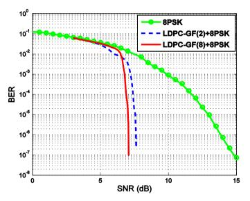
Figure 5. BER v.s. SNR of Ka Link.
