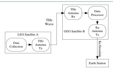
Figure 3. Block diagram of MODE 2 (LEO-GEO link).
