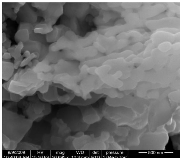
**Figure 5.** HR-SEM image of conventionally calcined powder at 900°C for 3 h.
