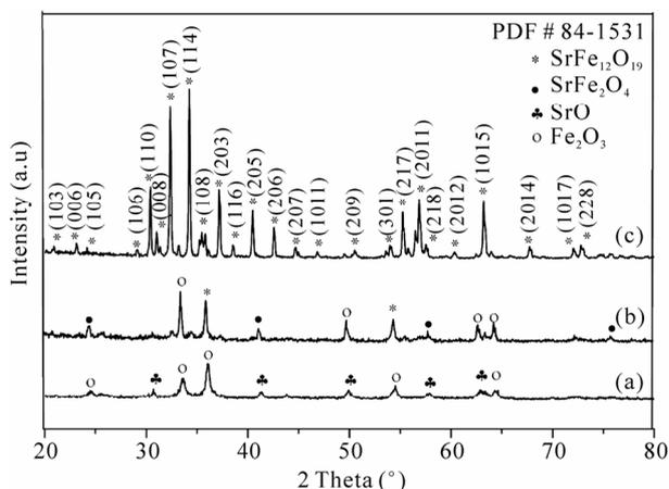
**Figure 3.** XRD patterns of the powders calcined at different temperatures: (a) 500°C, (b) 750°C, and (c) 900°C for 3 h.
