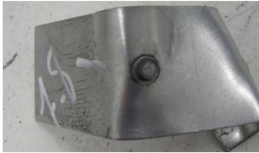
Figure 3. Coach-peel tested coupon.
