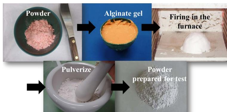
**Figure 1.** Preparation of diatomite extracted from alginate impression gel.
