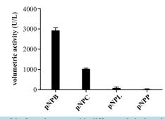
**Figure 3.** Volumetric activities of Trx-Lip for substrates with different chain length. pNPB: p-nitrophenylbutyrate, pNPC: p-nitrophenylcaprylate, pNPL: p-nitrophenyllaurate, pNPP: p-nitrophenylpalmitate; The highest activity was observed for pNPB hydrolysis.
