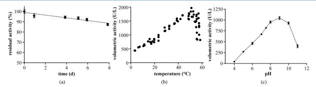
**Figure 4.** Biochemical characterization of Trx-Lip. (a) Stability of Trx-Lip in buffer, even after 8 days > 85% residual activity was observable; (b) Volumetric activity of Trx-Lip at varying temperatures, the temperature optimum is  $\sim$ 50°C; (c) Volumetric activity of Trx-Lip at varying pH values, the pH optimum was determined to be at pH 9.0.
