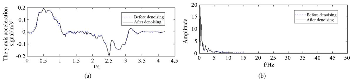
Figure 11. The waveform and spectrum diagram of de-noising before and after of y axis acceleration signal.
