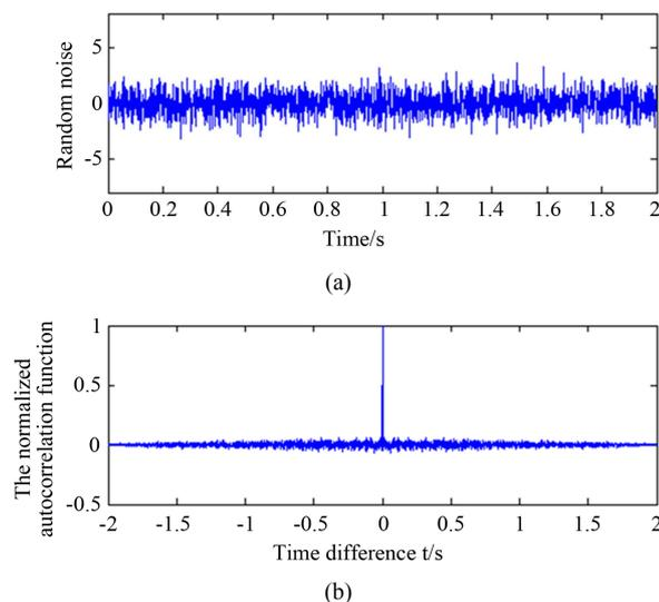
**Figure 4.** Noise and normalized autocorrelation function.
