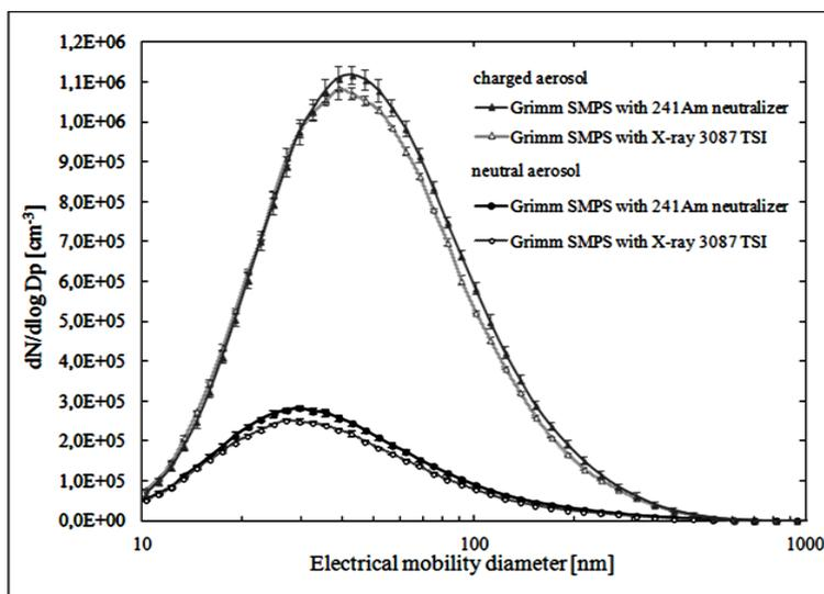
**Figure 2.** Aerosol size distribution for <sup>241</sup>Am and X-ray neutralizers (charged and neutral particles).
