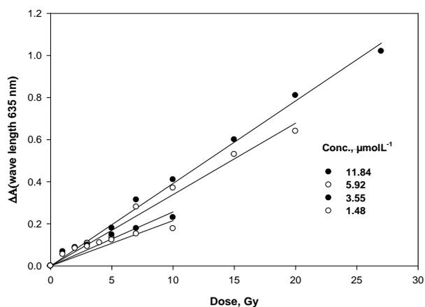
**Figure 3.** Linear dose response of the (TBO-gelatin) gel at 635 nm in the low-dose range of 1 - 30 Gy.
