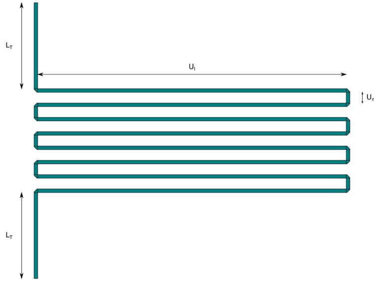
Figure 6. Simplified folded microstrip delay-line.
