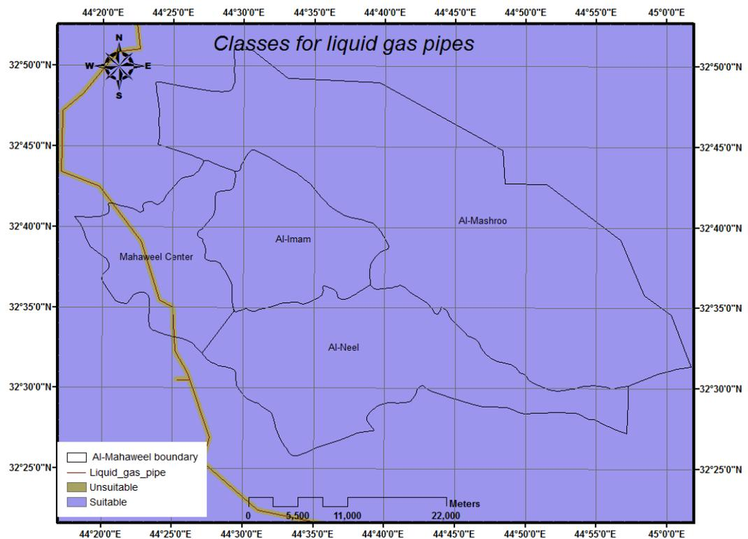
Figure 17. Classes for liquid gas pipes. \*Source for pipe lines: pipe lines company, Babylon, Iraq, 2012.
