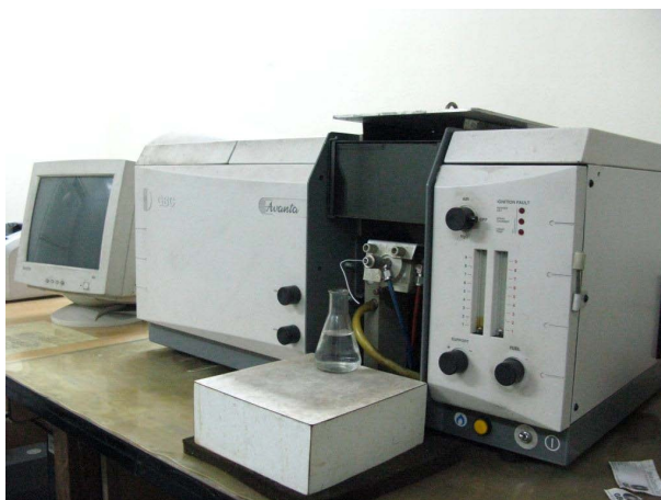
Figure 3. The Avanta GM FAAS used for the analysis.
