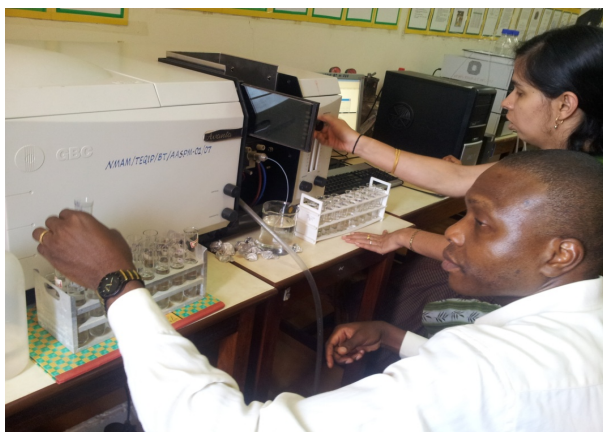
Figure 4. Determination of the trace elements in wastewater samples using the FAAS.
