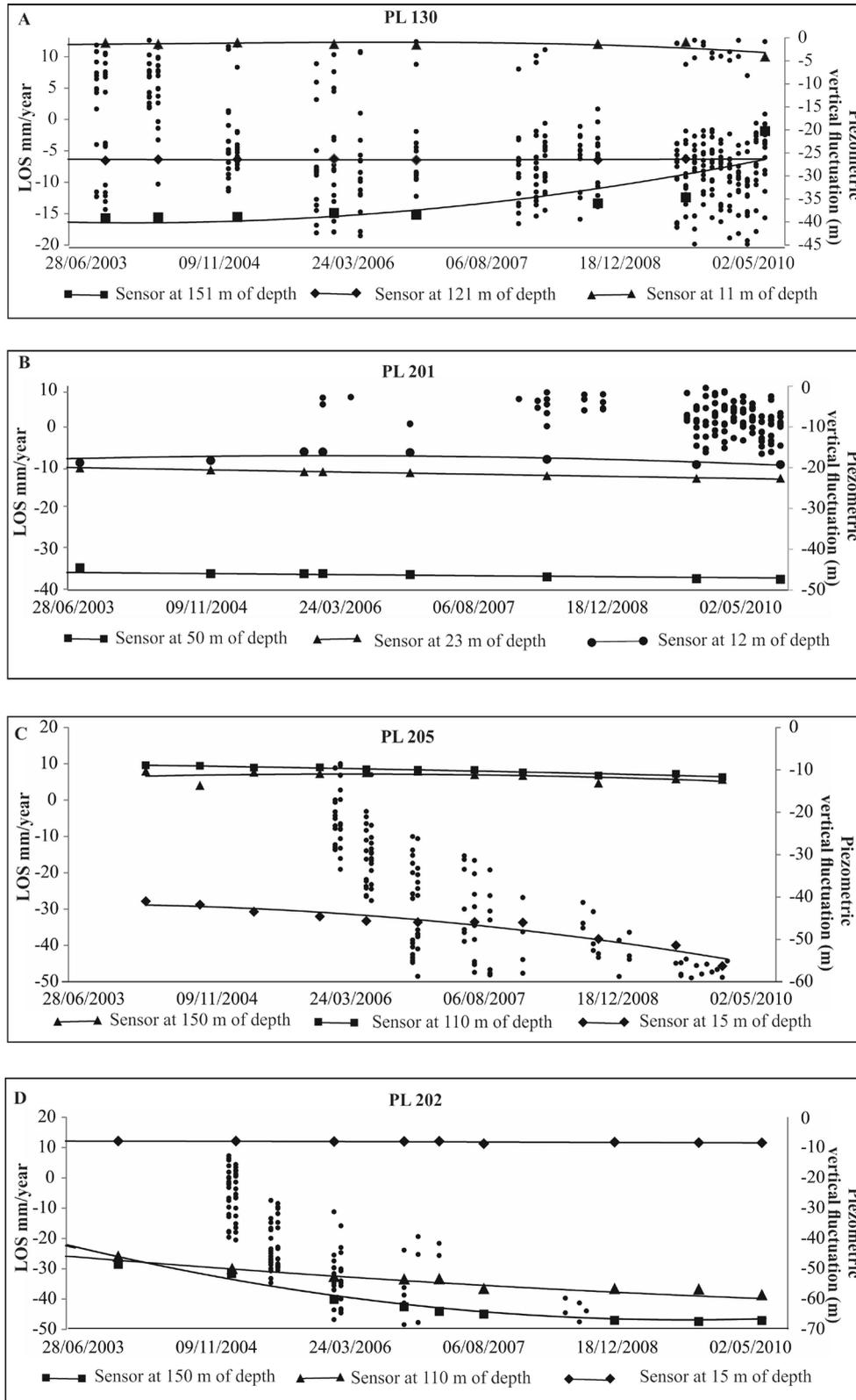
**Figure 5.** Graphics of the profiles along the selected windows (see Figure 4). The graphics show the historical relationship between piezometric data and the LOS map for the period 2003-2010. The multi-piezometers selected were PL-130 (A), PL-201 (B), PL-205 (C), and PL-202 (D).
