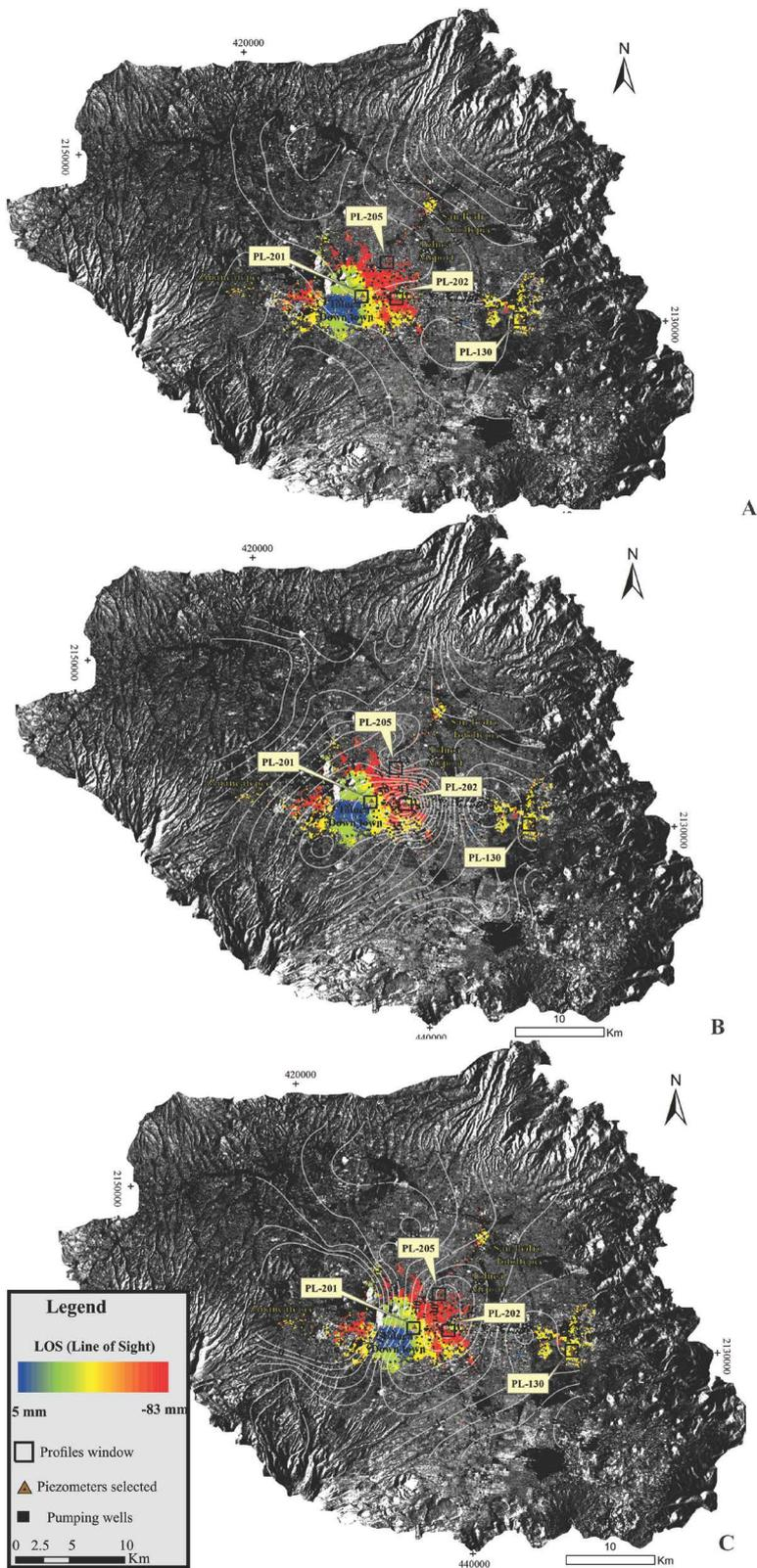
**Figure 4.** Distribution of PS with respect to isolines of maximum piezometric fluctuations for the period 1970-2010 considering only three levels of depth: 50 m (A), 100 m (B), and 150 m (C).
