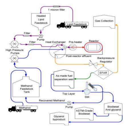
Figure 4. Process flow diagram of a biodiesel plant based on the Mcgyan process.
