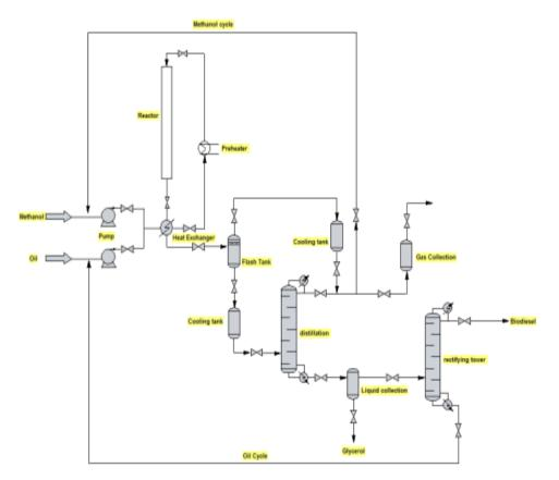
Figure 5. The route of production biodiesel by tubular reaction system.
