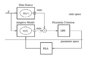
Figure 1. Unrealistic framework. *Legend*:  $\mathcal{X}$ —experimental condition; OPI—Original Performance Index; PAA—Parameter Adaptation Algorithm.
