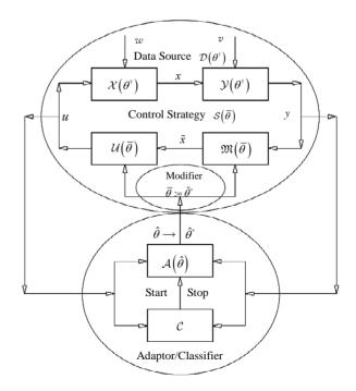
Figure 4. Adaptive stochastic control system structure.
