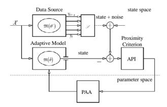
Figure 3. The API framework *Legend*: API—Auxiliary Performance Index.
