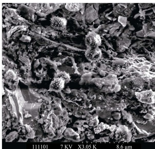
**Figure 5. Cross section SEM micrograph on sandblasted steel (Sa 2.5).**
