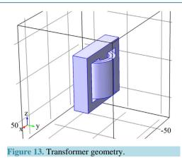
Surface: Magnetic flux density norm (T) Arrow Volume: Current density Arrow Volume: Current Density
