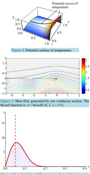
**Figure 6.** Irradiated heat diffusion curve for winding *x*.
