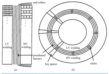
Figure 1. Transformer winding. (a) Side view; (b) Top view.
