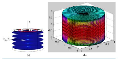
Figure 3. (a) Heat measure per unit of sectional conductor; (b) Total contribution of the generated heat for all electrical conductors.
