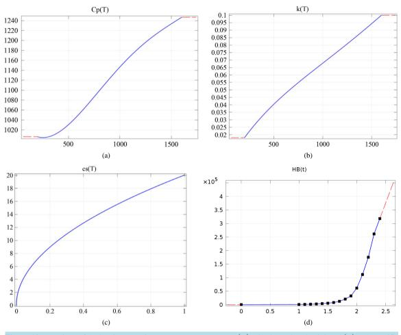
Figure 12. Functions of (a) heating capacity to constant pressure  $C_p(T)$ ; (b) thermal onductivity k(T); (c) specific heat  $C_s(T)$ , and (d) normal of magnetic field HB(t).
