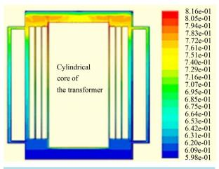
Figure 9. Temperature distribution due to the heat generation coming from windings-core.
