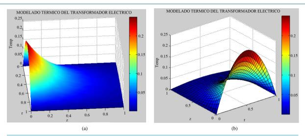
Figure 16. Idealized winding temperature distributions shaped by the specific heat and heating capacity to constant pressure curve (see the Figure 12(a) and Figure 12(c)).
