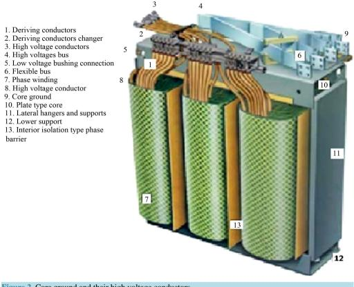
Figure 2. Core ground and their high voltage conductors.
