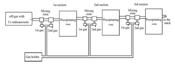
Figure 1. New decontamination set-up.
