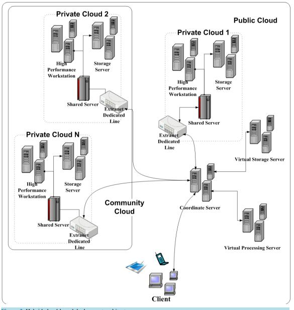
Figure 2. Hybrid cloud-based deployment architecture.
