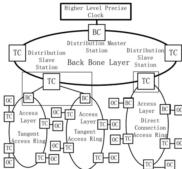
**Figure 2.** Wide-area multilayer correcting time network of unified distribution network.
