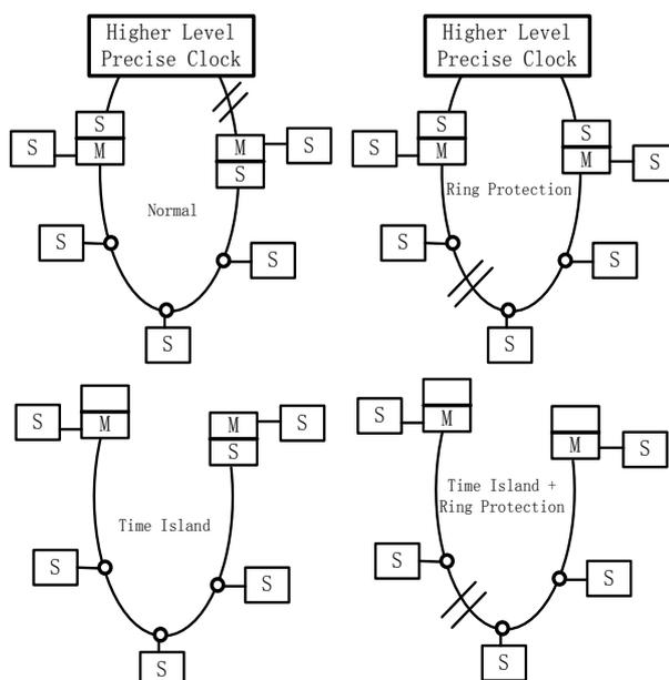
**Figure 3.** Four kinds of synchronization trees of direct connection access ring.
