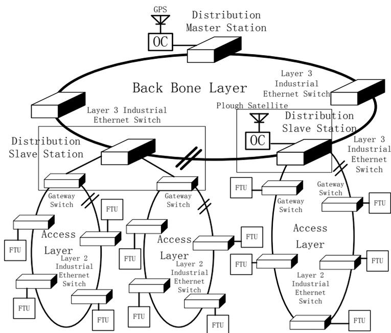
**Figure 1.** Typical topology of distribution network communication system based on industrial Ethernet.
