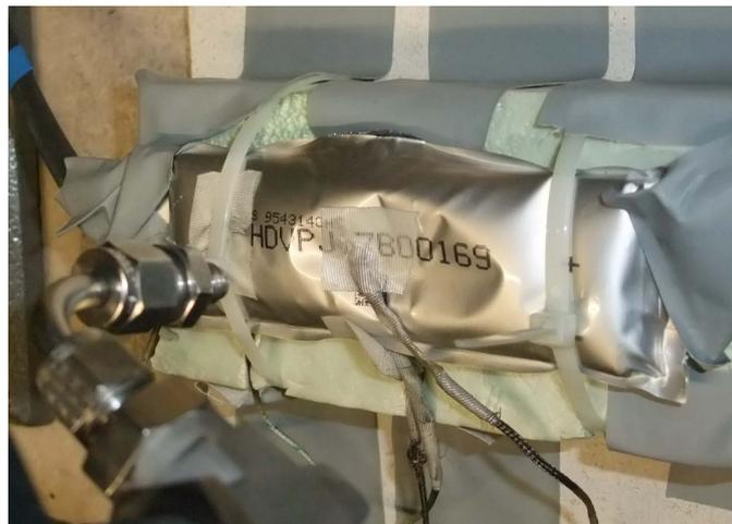
**Figure 8.** Cell after emergency cooling experiment. Cell inflated and the  $\text{CO}_2$  pulse resulted in a dented cell. No cell rupture occurred.
