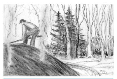
**Figure 6.** Charcoal production by the pit method was very labor-intensive and required 24-hour supervision by a collier (Charcoal sketch by artist Susan Styer).
