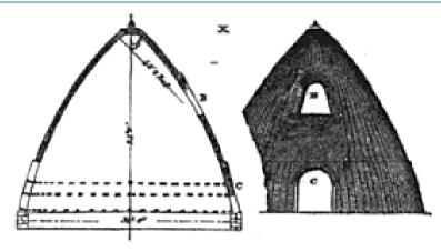
Figure 4. Conical charcoal kiln (Birkinbine, 1891).
