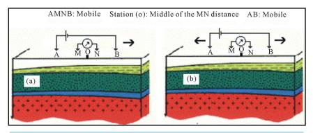
Figure 4. (a) Schlumberger electrical profiling, (b) Schlumberger electrical sounding.
