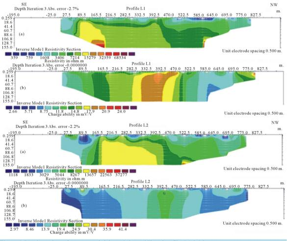
Figure 6. Pseudo-sections of apparent resistivity and chargeability of profiles L1 & L2.
