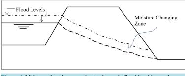
Figure 4. Moisture changing zone due to change in flood level in canal.
