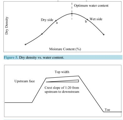
Figure 6. Top width section, crest slope, after [37].
